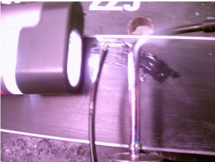
The Repair has been filled with the new plastic. Shown is the repair string, heating element and the new plastic that has not been shaved down.
