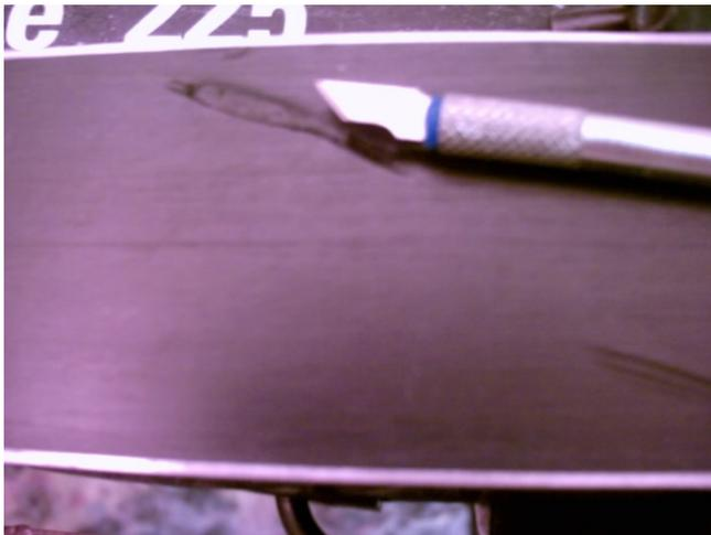
To fix this cut, two different plastics will be used. METAL GRIP is a Co-polymer plastic and adhesive mixed. It is rubbery and will adhere to the core fiberglass or metal edge.
