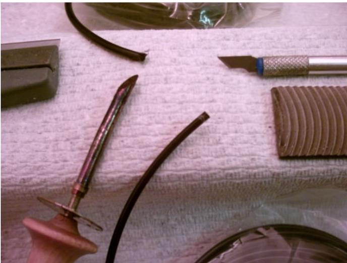
Use the wooden handle heating element to melt a piece of METAL GRIP and press it into the cut. Make sure to heat the plastic till it flows. Press into the cut to assure bonding to the core base. Leave space at the top of the cut for the P-tex repair string to be filled in.
